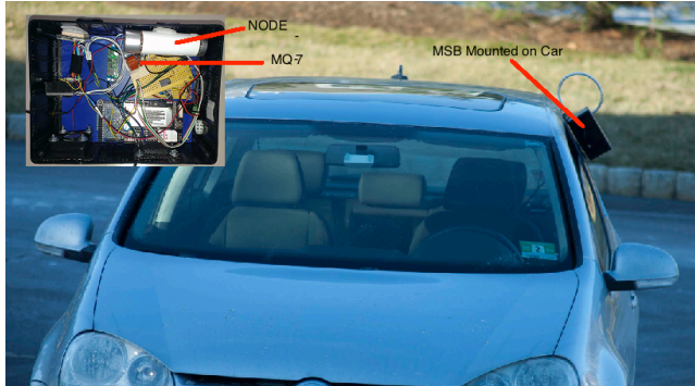
Figure 6 MSB Mounted on Car
