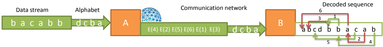
Figure 1: A first sends B the alphabet abcd then it sends the codewords of gaps between consecutive occurrences of a character. B decodes the gaps and uses them to refer to the characters in part of the stream having been already decoded. The reference stream is E(3)E(1)E(6)E(5)E(2)E(4) .
