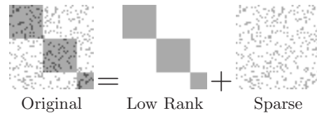
Figure 1: Decomposition of the evolution matrix in Eq. (5) into low-rank and sparse matrices.
